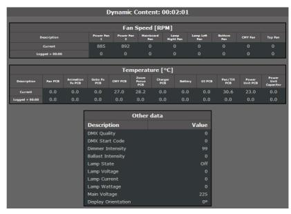
The example below in the **Dynamic Content** section, shows temperature data for the different sensors in the fixture. In the example, the fixture was powered on 3 hours and 15 minutes before the current temperature data was logged. Temperature change over time at 15 minute intervals can be followed in the table. If you wish, it can also be copied and pasted into spreadsheet software such as Microsoft Excel.
