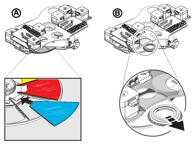
Figure 21: Color filter and gobo replacement
