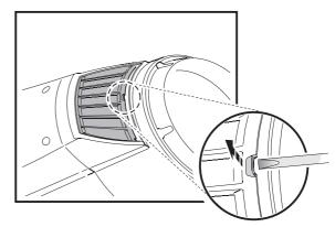
Figure 17: Removing head air filters
