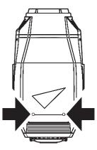
Figure 20: Head cover screws
