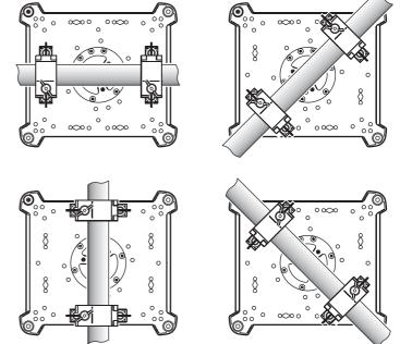
Figure 4: Clamp bracket positions
