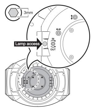
Figure 3: Lamp adjustment screws
