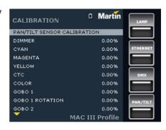
Warning! As soon as you exit pan/tilt sensor calibration, the head will move to its original position.
