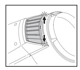
Figure 19: Reinstalling head air filters
