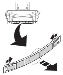
Figure 18: Base air filters
