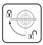
Figure 7: Locking 1/4-turn fasteners
