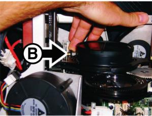
Figure 26: Moving the zoom/focus car fully forward
