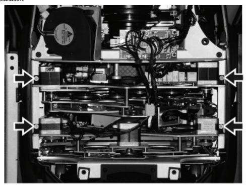
Figure 27: Module retaining screws
