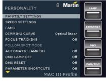
Pan range for pan limit purposes runs from  $0^{\circ}$  to  $360^{\circ}$  clockwise as seen looking at the fixture from the bottom of the base towards the yoke, as if the fixture was hanging downwards underneath you. Tilt range is  $+134^{\circ}$  and  $-134^{\circ}$  either side of  $0^{\circ}$ , which is the head straight up position with the front glass pointed directly away from the base.
