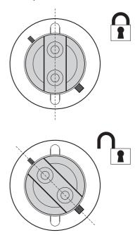
Figure 2: Lamp removal / refitting
