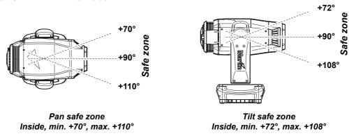
Figure 10: Pan/Tilt limit settings
