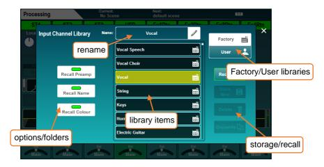
Factory libraries provide presets and are also used to recall different FX units or DEEP plug-ins. They are fixed in firmware and cannot be edited or overwritten.
