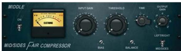
The Fairchild 670 tube compressor achieves record bids in high-end vintage gear auctions, due to its highly musical colouration, which makes it a classic in the history of compressors. Two small trimming potentiometers set the control side chain action, a six-step switch determines the timing, and the two large Input and Threshold knobs adjust the levels.
