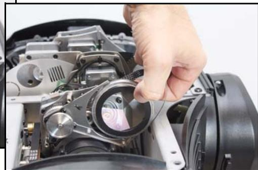
**Figure 19: Removing the rotating prism**
