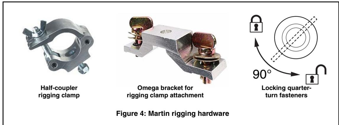
3. See Figure 3 on page 7. Align the first clamp and bracket with 2 mounting points in the base, and engage both the clamp bracket's quarter-turn fasteners in corresponding sockets in the base. See Figure 4. Turn the levers on the quarter-turn fasteners a full 90° clockwise to lock. Repeat for the second clamp.
