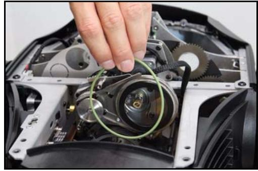
**Figure 18: Removing the prism drivebelt**
