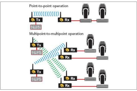
Fig. 1: Point-to-point operation versus multipoint-to-multipoint operation
