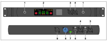
Fig. 16: Connectors and ports of ProBox F-2500 (Upper picture: front panel; lower picture: connector rear)
