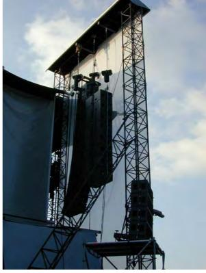
Figure 91: Stacked V-DOSC offstage fill system (Radiohead, Oxford 2003, sound design - F. Bernard)
