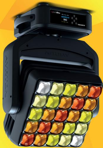
With 900 Watt of total power, the versatile MAGICPANEL™FX has 25 next-generation RGBW high-power LED emitters and an active phase-change liquid cooling system using a heat pipe for intensive use in “wash light” mode. The continuous, unlimited, rotation on pan and tilt, first introduced on the legendary MAGICPANEL™602 in 2013, is standard. MAGICPANEL™FX has serial connectivity and can be controlled using DMX-RDM, ArtNet™, sACN or wireless CRMX TiMo RDM by LumenRadio™.
