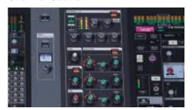
The Yamaha Selected Channel concept is familiar to and highly regarded by most seasoned sound engineers. The RIVAGE PM5 Selected Channel Section consolidates an essential group of physical controls in a compact section that allows fast, intuitive operation. In combination with the touch-sensitive display panels the Selected Channel Section provides even more comprehensive control for extremely efficient operation.
