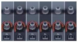
The RIVAGE PM10 and PM7 consoles feature two encoders for each channel; channel strip encoders that can be assigned to five different functions, and screen encoders that control the corresponding parameter on the adjacent display panel. Physical controllers are simply unbeatable when it comes to hands-on control, so the availability of two encoders per channel gives the PM10 and PM7 an operational advantage.
