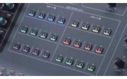
24 physical User Defined Keys can be assigned to directly recall any functions the engineer will be using frequently, for fast one-touch access in front-of-house and monitor applications.
