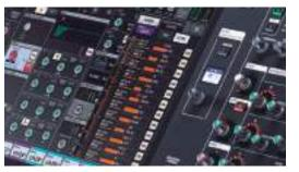
Setting up sends is an important part of just about any live mixing workflow. In addition to the familiar Sends on Fader function, send levels can be controlled from the Send / User Defined Knobs. Send levels shown on the display panels where they can also be adjusted via touch control. This expanded range of control choices greatly enhances convenience and versatility when setting up and tweaking sends.
