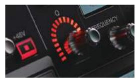
Great care has been taken to ensure that operational feedback to the engineer is always clear and consistent, so that appropriate mixing decisions can be made. Even the "horseshoe ring" indicators surrounding the multi-function encoders at the top of the fader strips have been carefully designed so that all segments remain fully visible from the engineer's viewing position. Every detail counts, especially in live mixing situations.
