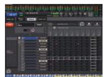
The Overlay filter can notably enhance the usefulness of the console's scene memory. It can be "overlaid" on a current mix to apply offsets to the fader levels and mix/matrix send levels independently from scene recall. This can be useful when an unplanned performer change occurs, for example, facilitating a temporary, relative level adjustment that can be instantly returned to the original level. The
